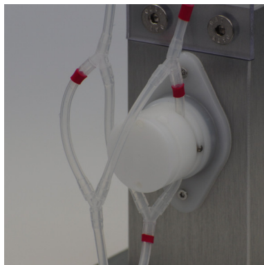
Figure 22 – Insert the tubing coming from reservoir B into the right side slots. The marked tubing goes in the rear slot.
