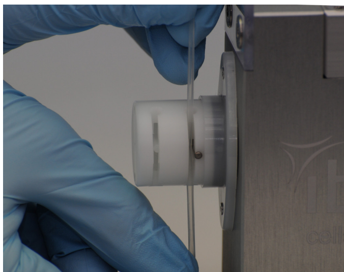
Figure 25 – Move the tubing up and down while stretching for easy placement into the valve slots.
