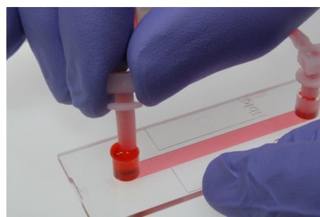
Figure 31 – Connect the second Luer adapter to the \mu -Slide.
