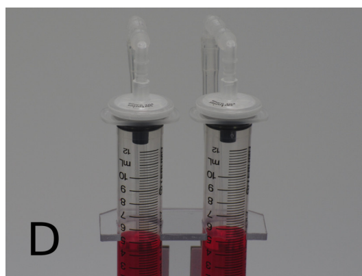
Figure 27 – Fill the syringe reservoirs with medium to equal levels and connect the filters to the reservoirs again.
