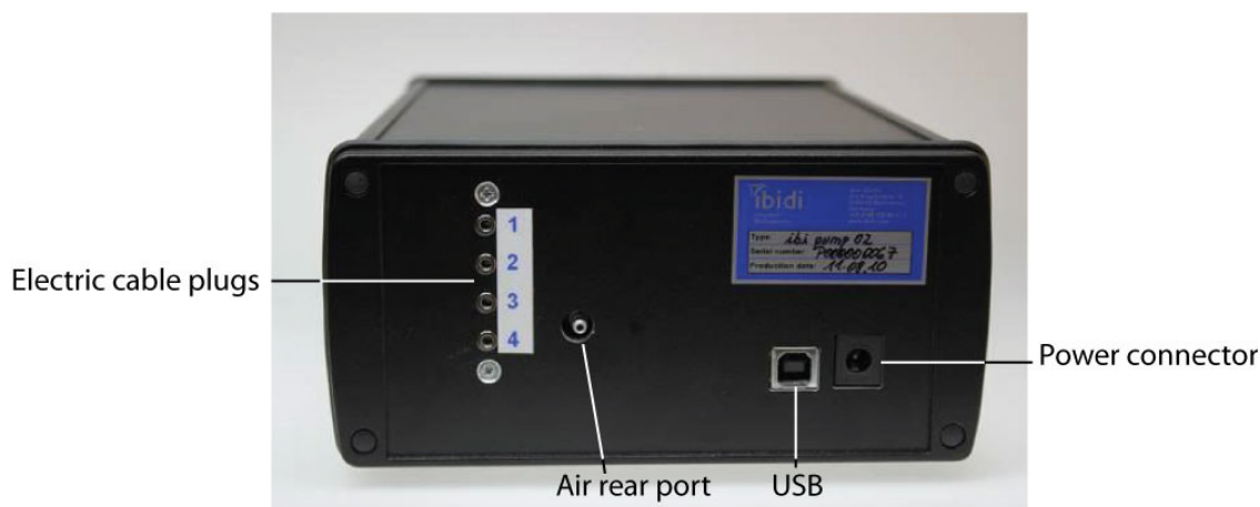
Figure 2 – Rear view of the ibidi Pump with air rear port, connections for the USB, power supply port, and electrical cables ports to the Fluidic Units.
