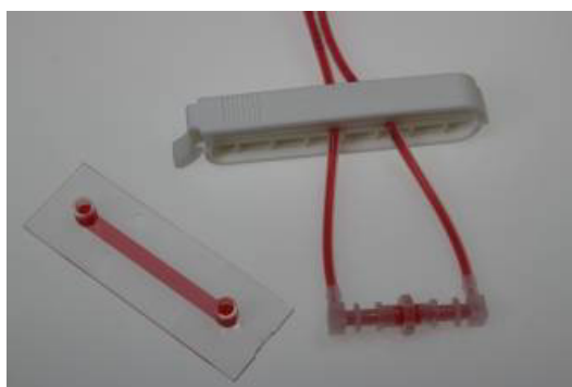
Figure 29 – Clamp the tubing before opening the Female Luer Coupler of the Perfusion Set.
