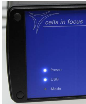
Figure 12 – LEDs on the pump’s front panel indicating the connected USB and power supply.
