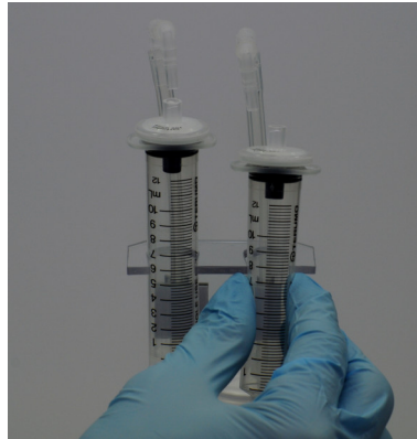
Figure 21 – Squeeze the reservoirs for insertion into the holder.
