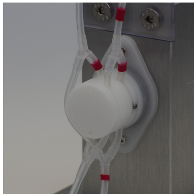
Figure 23 – Insert the tubing coming from reservoir A into the left side slots. The marked tubing goes in the rear slot.
