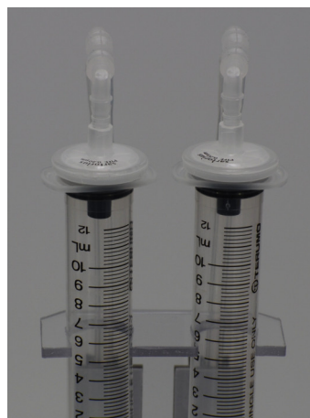
Figure 26 – Connect the filters of the Perfusion Set to the Fluidic Unit tubing.
