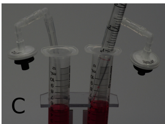
Figure 27 – Fill the syringe reservoirs with medium to equal levels and connect the filters to the reservoirs again.
