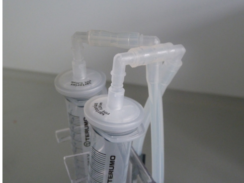
Figure 50 – Cross the tubing on top of the reservoirs to test if the problem is with the Perfusion Set or in the valve block (valve 1).
