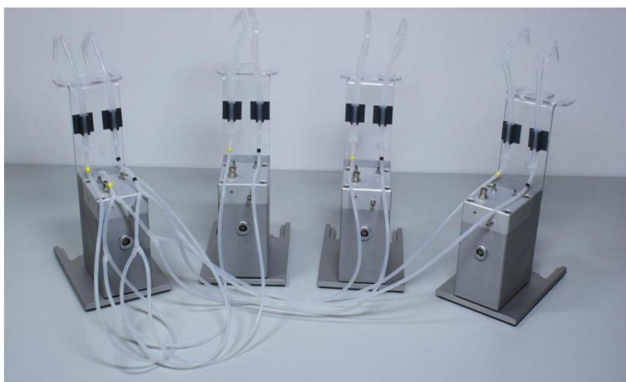
Figure 37 – Oscillatory flow setup with four Fluidic Units (one master and three slaves).
