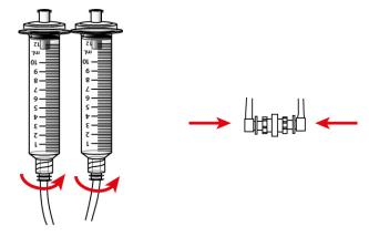
Check the tightness of the connections!
