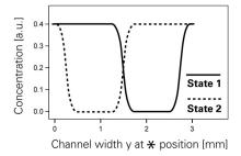
All flow rates should be adjusted in a way that the point of inflection of the sigmoid is at identical position in state 1 and state 2.
