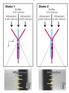
Concentration profiles can be visualized by using a fluorescent dye e.g. rhodamine. Switching time between state 1 and state 2 can range from seconds to hours, depending on the speed of the cells' response.
