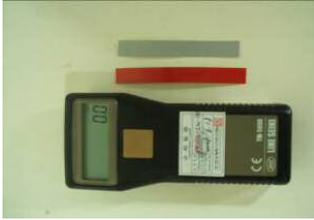
1. Prepare a RPM speed tachometer (hand tachometer) and fluorescent light tape.
