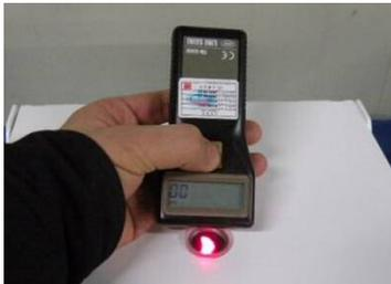
3. Set the specific rpm and start the operation.
