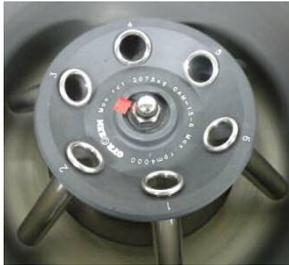
2. Attach some fluorescent light tape on a grip of a rotor lid.
