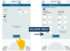
The Gilson Service button is accessible from Gilson Service representatives only by entering a unique PIN code, specific to Gilson. Complementary information can be filled in this menu when maintenance is done.
