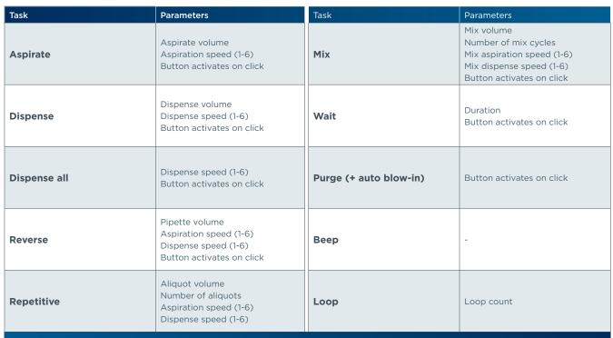
The activate on click toggle enables the execution of a task automatically or when the pipetting button is pressed. When "Activate on click" is selected, the task will start only when the pipetting button is pressed. When tasks are done automatically, "(Auto)" will appear after the name of the task on the screen as a reminder.
