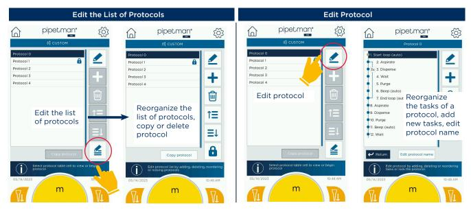
If Admin mode is enabled or if protocol is locked: touch the padlock icon and enter the PIN code
